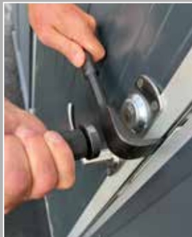
Quick entry with “hammer” part on Outward going doors.
